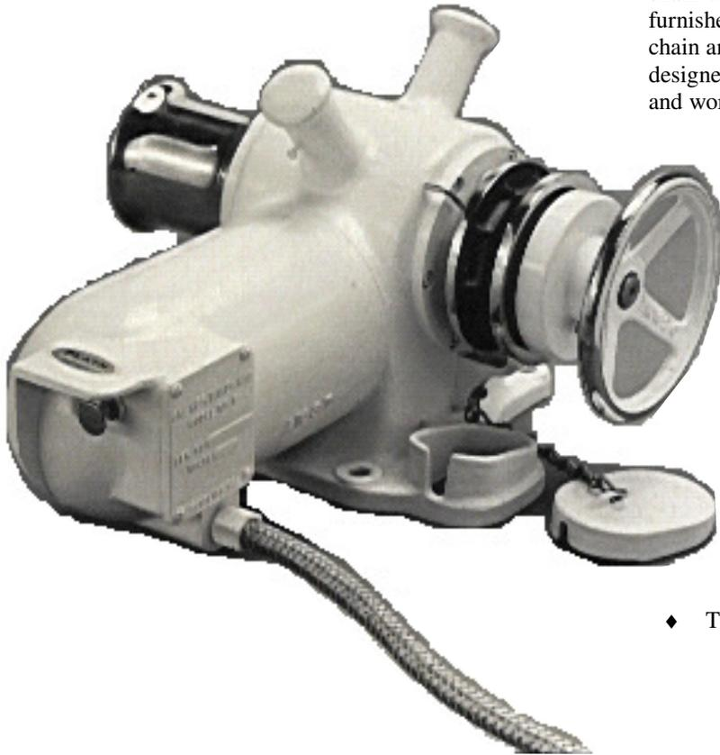
As on all PLATH Power Windlasses, power is applied to the chain wildcat through a cone clutch, which is also used as a brake when dropping anchor. The rope gypsy will turn independent of chain wildcat. An emergency handle operating device is furnished for use in case of power failure. Deck pipe will handle chain and line with thimble. The Model No. 5 windlass is designed for use with chain and/or rope on both pleasure craft and work boats.
